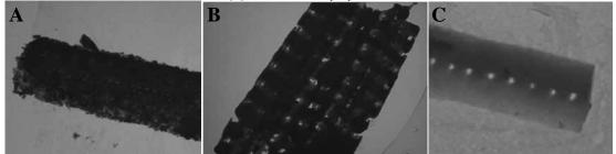
Fig. 2. TEM. A: Magnetized diatom frustule. B, C: Bare frustule/girdle band protected from magnetization.
